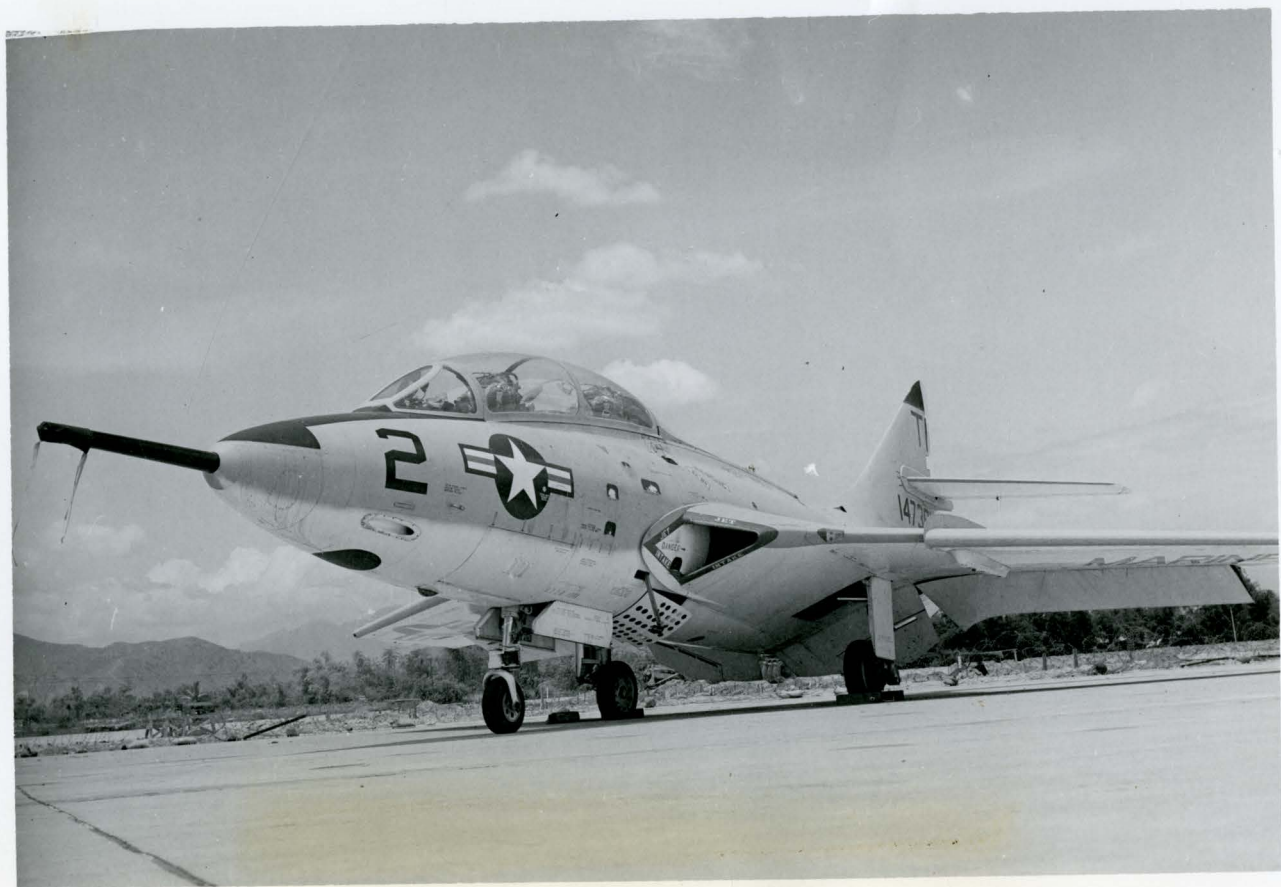
The TF9J "Cougar" is a single jet engine, two seat (tandem type) aircraft utilized as a tactical airborne coordinator.
