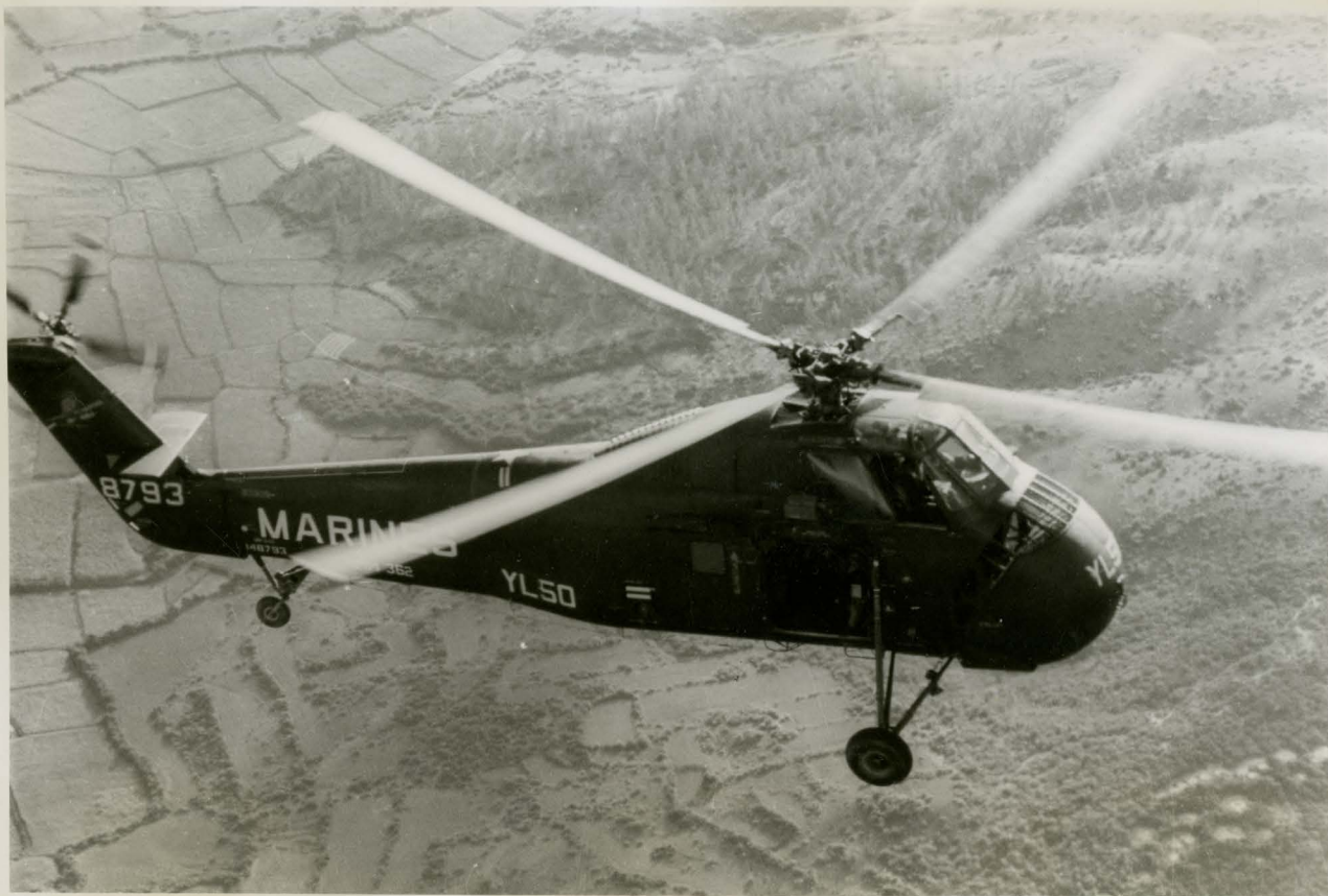
The UH34D is a single engine helicopter designed for transportation of cargo and personnel including aeromedical evacuations.
