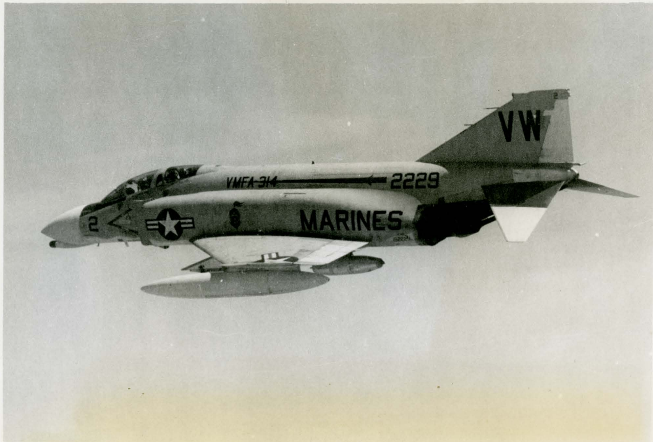
The F4B "Phantom" is a tandem type two seat supersonic fighter attack plane equipped with twin jet engines.
