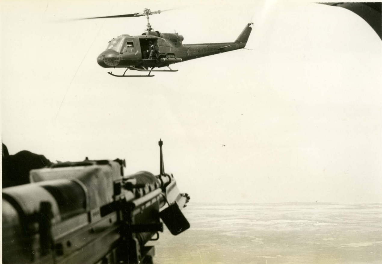
The UH1E "Huey" is a jet turbine helicopter, designed for utility use. A Gunship version supplies close air support.
