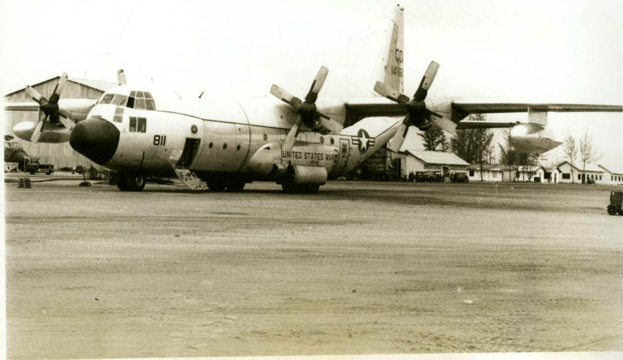
The KC-130F "Hercules" is a four engine, long-range aircraft designed to provide inflight refueling or transportation of personnel or cargo.
